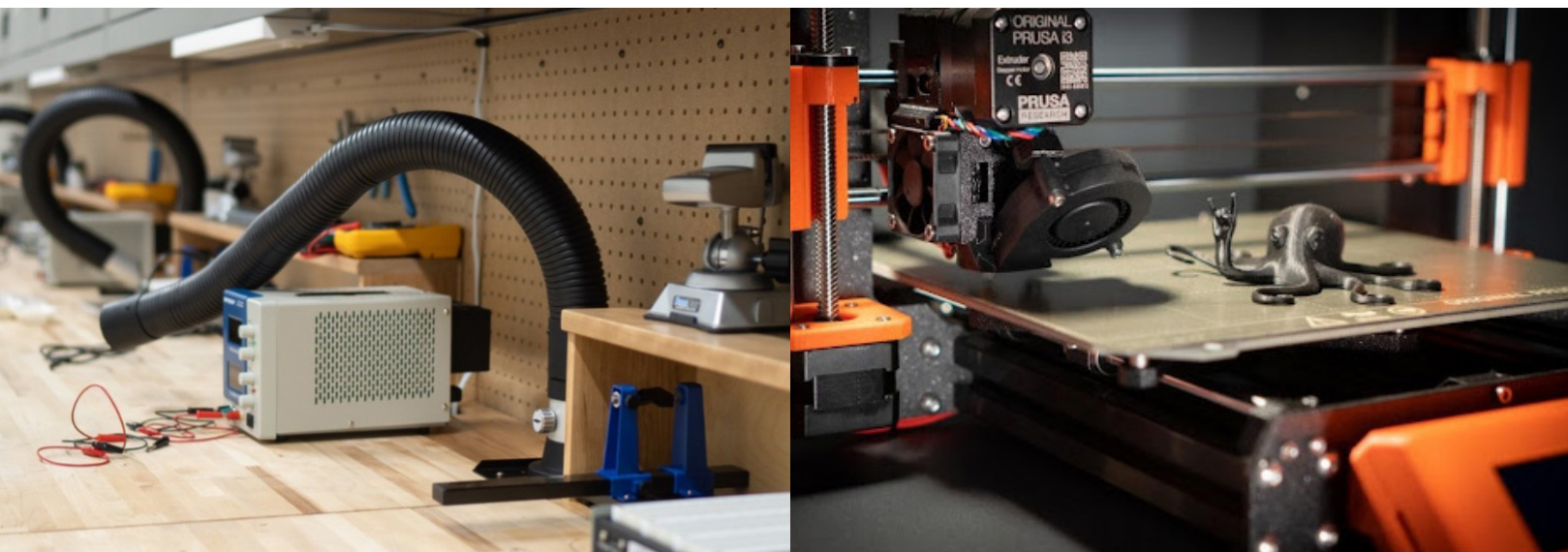
(Left) Work stations are setup on the electronics work bench that is outfitted with the necessary equipment for performing design and development or troubleshooting of electronics. (Right) There is a printing cabinet filled with Prusa filament style printers. These printers will be used for creating prototype components and are part of the additive manufacturing capabilities of the iLab.
